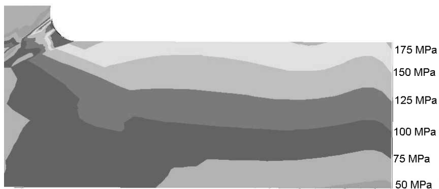
Figure 4- Stresses in the legs calculated by Finite Element Method
